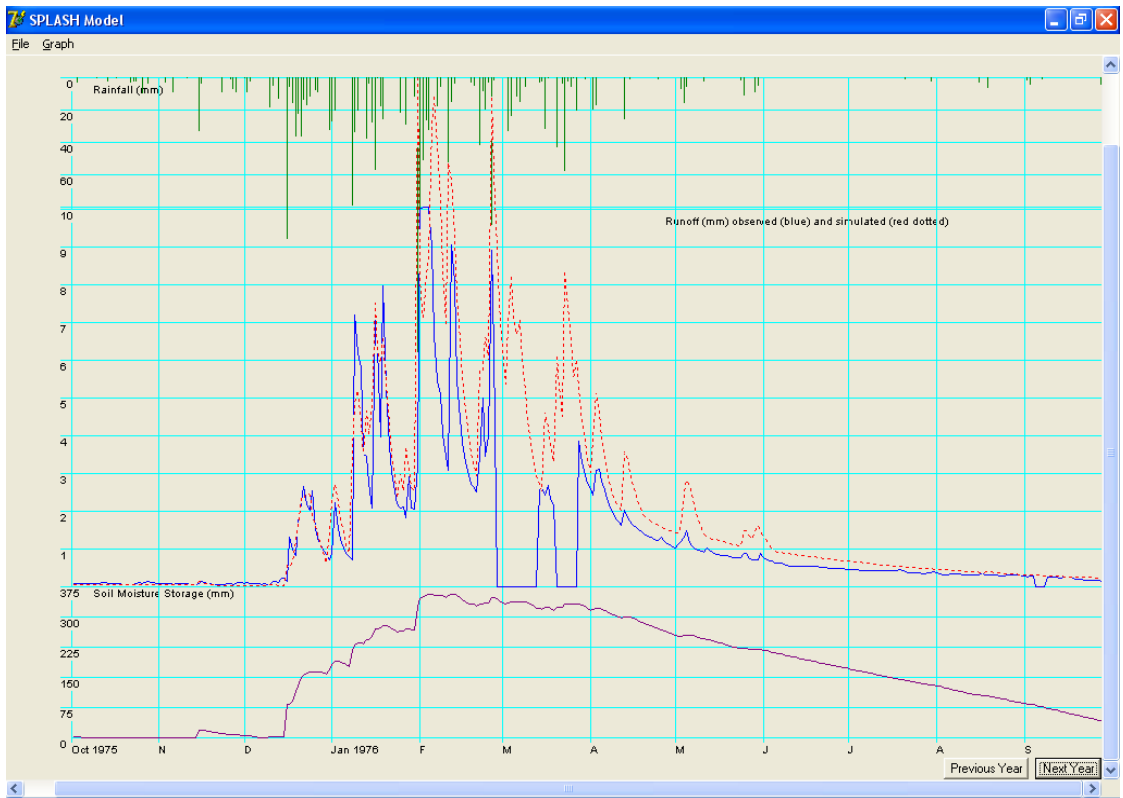
Figure 3: Weir / calibration table limit exceeded early in February 1976. Note the in-filled flows during Feb/Mar 1976
